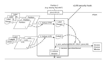
Figure 4: Security hook guarding the joining of a vLAN.
