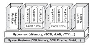
Figure 1: Hypervisor architecture augmented with security services running in an isolated partition.
