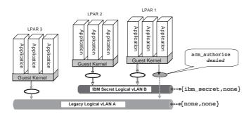
Figure 7: Multi-level secure vLAN based on sHype.
